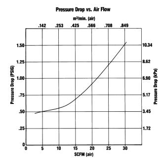
3/4" Orifice, O-ring Free Design, Machined
