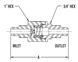
$\dagger$ Tube connection includes Integral Ferrule nuts. Also compatible with Quikgrip $^{\circ}$  fittings. See page 250 for information.
